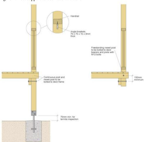
Figure 4: Post support to deck sub-structure
