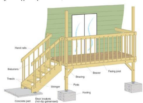
Figure 1: Typical layout of stairs, handrails and balustrades
