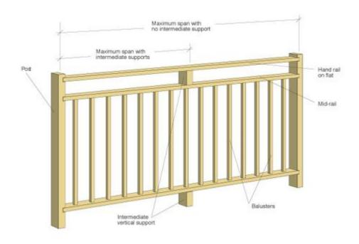
Table 4: Handrail sizes and maximum spans
